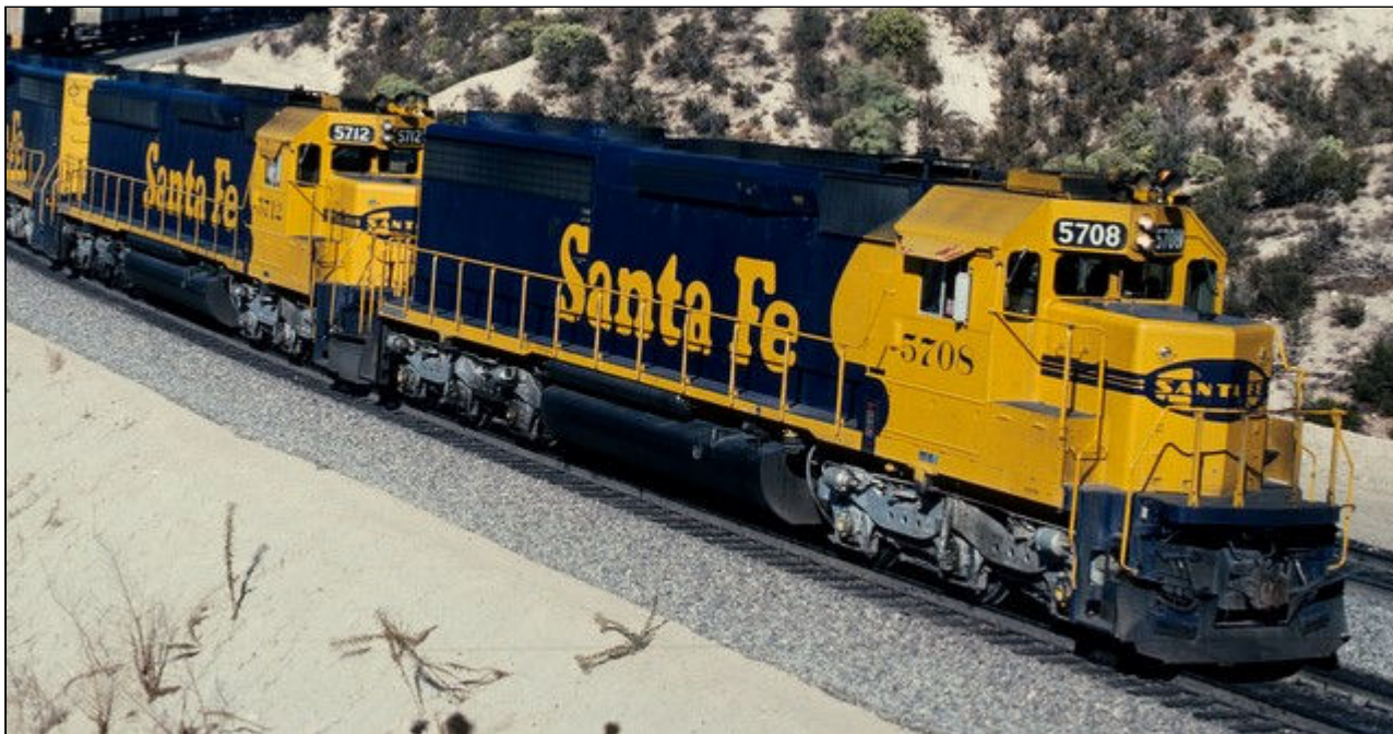
Above - This closer view of ATSF SD45-2s 5708 and 5712 clearly shows the different style radiator air intake grilles on the 5708 and 5712. The 5712 has the experimental inertial type and the 5708 has the standard wire-screen type. ATSF 5706, 5707, 5712-5714 (5 units) were delivered with the EMD experimental inertial radiator fan intake grilles. Also note the Sinclair radio antenna, coupler lift bars with loop, and location of the vertical air vent toward the rear of the cab below the cab window on the engineer's side. Summit, CA 12-7-75. - Kodachrome by Ralph Back
