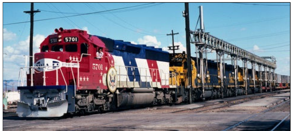
Right - ATSF SD45-2 "Bicentennial" 5701 on the point position of the westbound 198 Train Super C waits at the Needles fuel rack as other SD45-2's in the consist get fueled. The 5701 was rebuilt to SD45-2B 5514 in November 1987 and was on the BNSF roster as BNSF 7508 until renumbered BNSF 6523 in December 2006. Needles, CA 3-12-75. - Steve Patterson, Ralph Back collection
