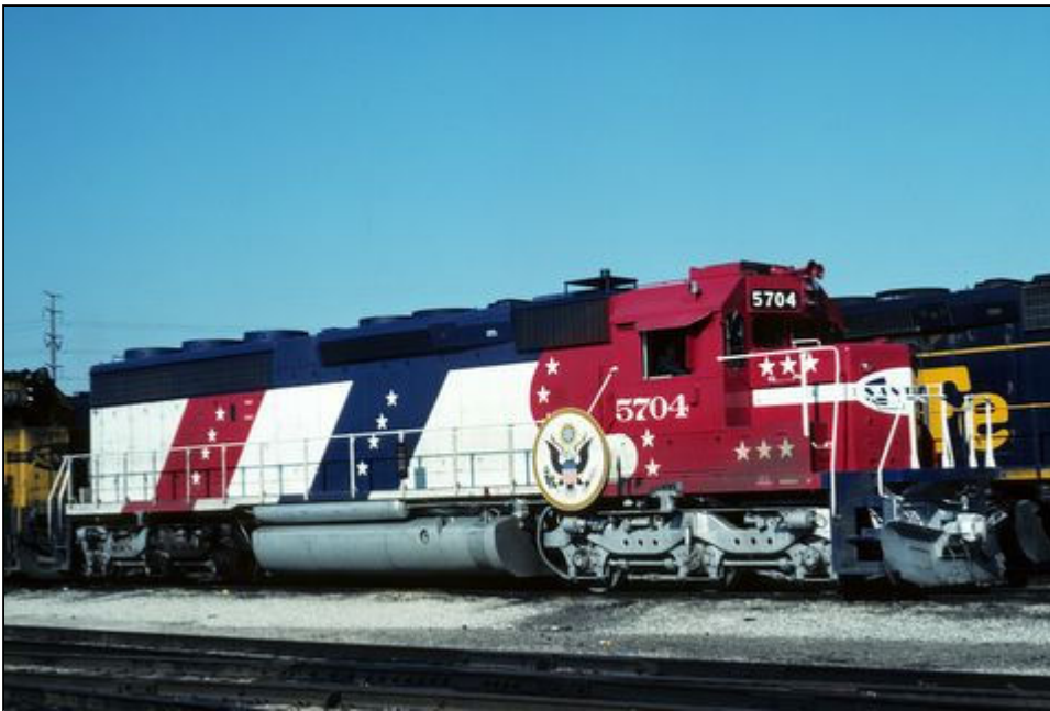
Left - ATSF 5704 was the last SD45-2 to be painted in the "Bicentennial" scheme in January 1976; and was rebuilt to SD45-2u 5834 in September 1986. ATSF 5834 is on the BNSF roster as BNSF 6484. Chicago, IL 4-10-76. - Kodachrome Ralph Back collection
