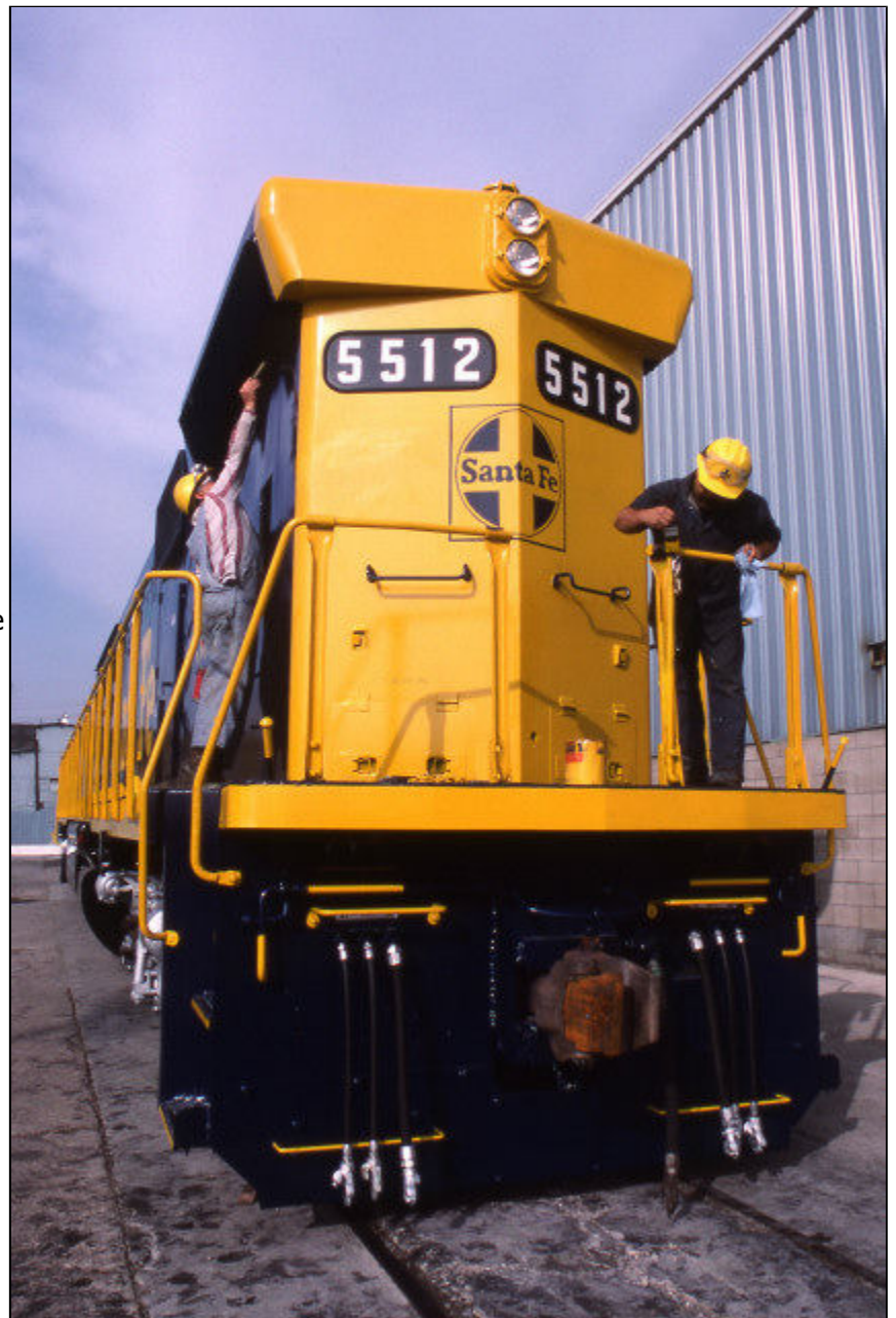
Right - ATSF SD45-2B 5512 has just been released from remanufacturing and two Santa Fe employees are touching-up its new paint job outside Santa Fe's San Bernardino Shops in October 1987. Note the full-width front anti-climber and the straight coupler lift bars. - Kodachrome by Mike Martin
