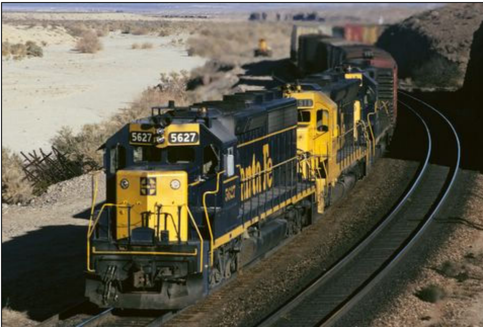
Left - ATSF SD45-2 5627 displaying its as delivered appearance in the then standard blue/yellow stripe scheme with dark blue Santa Fe cross herald. The 5627 was one of the units delivered without air-conditioning, and now has its horn mounted low at roof top level. ATSF 5627 was remanufactured to ATSF 5857 in April 1987 and was on the BNSF roster as BNSF 6506 until retired in May 2002 and sold to NRE. Ibis, CA 1-27-74. - Steve Patterson, Ralph Back collection
