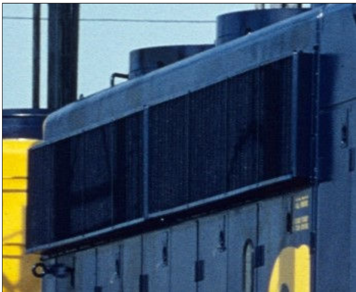
Close-up of ATSF SD45-2 5714's EMD experimental built-out EMD inertial radiator fan air intake grilles.
