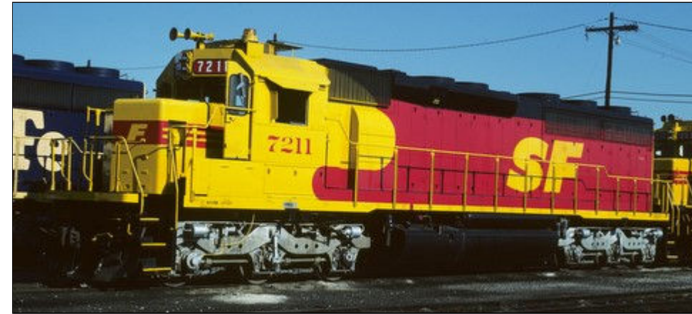
Left - SPSF SD45-2u 7211 was remanufactured in April 1986 from SD45-2 5685 from the second SD45-2 order, and now has Sinclair radio antenna, single fuel filler and no nose classification lights. The "home road" SF initials on the Conductor/Fireman's side were positioned toward the rear of the long hood with the F under the radiator grille. ATSF 7211 was renumbered ATSF 5811 and was on the BNSF roster as BNSF 6461 until retired in July 2004 and sold to NRE. Phoenix, AZ 6-26-86. - Kodachrome Ralph Back collection
