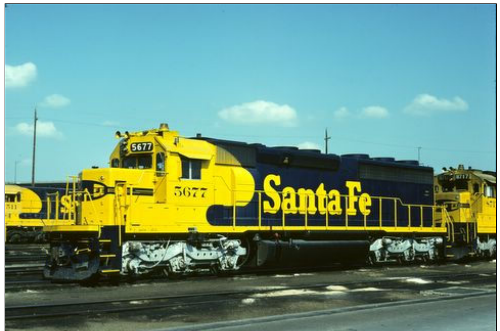
Right - ATSF SD45-2 5677, at Kansas City, KS 9-4-78, has been repainted and now has yellow step tread edges and yellow front anti-climber face, "Santa Fe" lettering style, and silver painted trucks. The 5677 was remanufactured to SPSF SD45-2u 7208 in March 1986 and later renumbered 5808, and was on the BNSF roster as BNSF 6458. In February 2008, the 6458 was repowered with a 16-cylinder 645 engine, designated a SD40-2R, renumbered 7953 and painted in the new BNSF Heritage scheme. - Kodachrome Ralph Back collection
